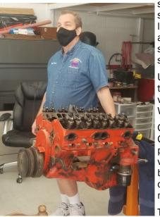
see an engine on a stand so the action of the cam, lifters, pushrods, rocker arms and valves could be seen relative to the crankshaft balancer.
