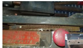
or two of Kroil penetrating oil took care of. Some areas of rust, mostly on the underside area, were cleaned up, and I decided to take a few components out for powder coating (those items associated with the vacuum blades and cover).
