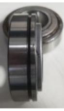
should press it out from the bottom. With the assistance of a friend's press, the drum easily came out of the housing, and the bearings came off the shaft easily as well. Now I could start the search for replacement bearings.
