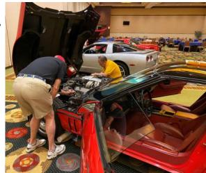
First things first, I attacked the engine issue. After replacing the fuel regulator valve and valve seals, the engine ran smooth and no sign of oil smoke. A tune-up with new plugs, wires, rotor & cap, oil change and filters, as well as new valve covers, helped to clean up the engine bay. Replacing the aftermarket wheels with factory wheels, new tires and new brakes all around improved the ride a great deal. A weekend spent
