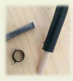
In order to remedy the collapsed hose, I removed it and inserted a wood dowel that was just a bit larger than the inside diameter of the hose. I also stopped by my local Ace-Hardware store and picked up a two (2) inch long steel springs. I left the dowel inserted and warmed the area with a hair dryer set on high. This helped to ease the collapsed area a bit. See Photo #2 at left for an example.
