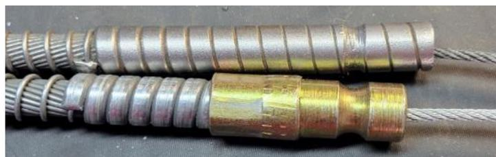
Essentially the end of the cable doesn't match the diameter of the original cable, as shown in the picture at right (original on top). The increased diameter forces you to expand the welded-on bracket to the point where inserting the bolt takes more effort than it should, and looks like it was something forced versus something intended.
