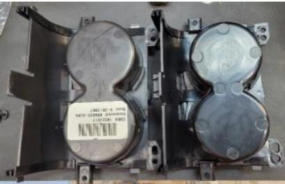
Now that NCRS is judging C6s, it may be important to make sure the replacement part looks and functions as original. In this case of the cup holder, the visible portions are identical. However, the backside differs in manufacturing markings and labels (not that anyone would see those). I mention it here as there may actually be original-type units available for likely a higher price. The picture at left shows the original (left) and replacement.
