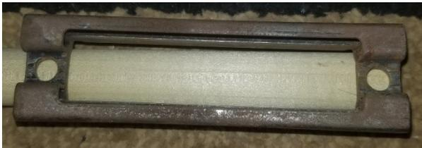
using a 3/4" wooden dowel (pic at left). Using the original mount as a template, I cut the dowel to length and marked the locations to drill holes for the allen head retainers. Picture at right is the final result. Now I needed to order the actual belts, and make a more permanent mount using the metal rod.
