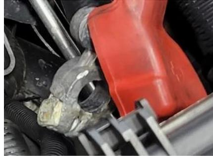
The solution at the time was to cut off the connector, strip back the wires, and install a universal connector as shown on left.
