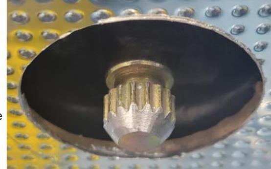
replacement regulators and I found that handle crank would not completely seat and thus the retainer clip would not engage. After examining the differences between an original regulator and the replacement it became apparent that the chamfer on the original was more pronounced. Using this tool resolved the problem. The photo at right shows the result.
