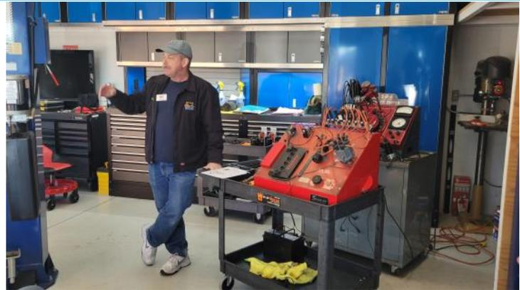
I showed many components of the two systems including how to diagnostically check each component. With a Snap-On ignition simulator, a full ignition system was operated and showed how the system works including a battery, ignition switch, starter solenoid, ballast resistor, ignition coil, distributor plus 8 spark plugs and wires. While spinning the distributor, we discussed how to check voltages on the various components was shown.
