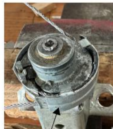
Fabricated Collar with Retainer Tabs J.B. Welded in place
