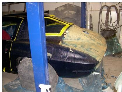
Now to the repaint. Going with the original color, Daytona Blue. In the series of photographs, it starts with taping off chrome, shielding tires, removing doors, and hood etc. and then applying the stripper. Messy and smelly are understatements. Protective clothing, breathing equipment strongly suggested, read mandatory.
