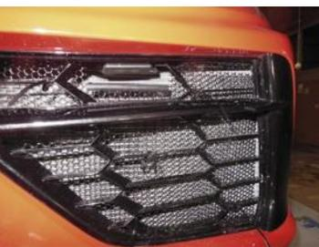
The front radiators get dented easily because they are near the road surface and they are a soft alloy. The race teams probably replaced them every other race, depending on the air flow loss. To avoid this expense, I recommend installing small mesh screens behind the factory grilles. Several vendors have these for sale, and the installation is not very difficult.
