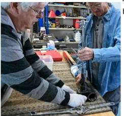
The disassembly is quick and easy. Removing the races and needle bearing assemblies is straight forward if you have the appropriate tools and exert a lot of force.
