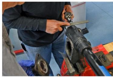
Once this adjustment was completed, the side cover was installed and the rebuild was complete.
