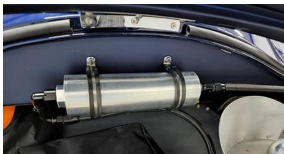
The Vapor Trapper is manufactured using 6061 billet aluminum, and is also rechargeable, meaning the charcoal contents can be replaced when they eventually become saturated. It is made to be used on all cars, trucks, hotrods, boats and everything in between! This will be the last charcoal canister you will ever need for your vehicle!
