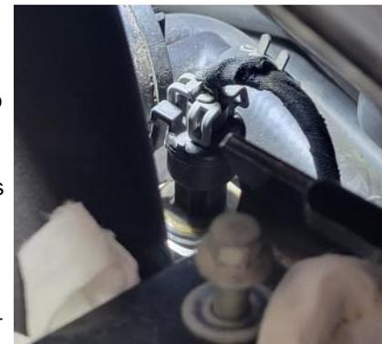
The picture below right shows the socket setup I used. The socket itself was just deep enough to ensure that it would catch the hex body of the sensor, but short enough to allow it to be slipped in and the over the sensors electrical connector.
